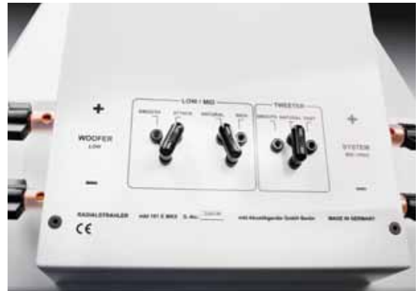
Jumpers allow the 101E’s tonal balance to be subtly altered.
