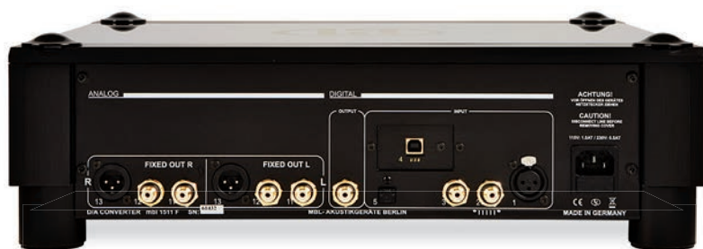
ABOVE: Two coaxial, one optical (S/PDIF) and XLR (AES/EBU) digital inputs are joined by a USB port. There is one coaxial digital output but a total of two single-ended (RCA) and one balanced (XLR) audio output. Input sample rates are limited to 96kHz
