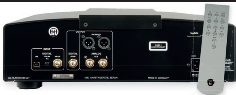
ABOVE: There are three 24/96-capable digital inputs: USB and S/PDIF via RCA and Toslink. Balanced (XLR) and single-ended (RCA) outputs are provided alongside a coaxial S/PDIF output. Remote controls complete MBL system
